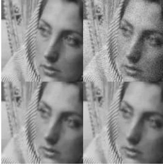
Figure 5.20: Qualitative denoising results for image barbara . From top-left, clockwise: original, noisy, TSITD denoised, BITD denoised.
