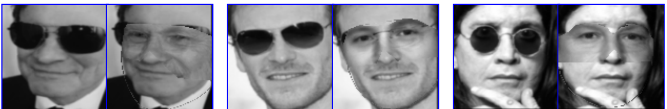
Figure 10: Original image ( left ) and reconstruction using our proposed method ( right ) when using automatically detected occlusion masks.
