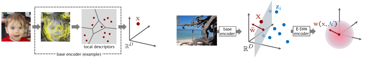
Figure 1. Principle of E-SVM visual encoder. (Left) Given a generic visual encoder, like BoW, Fisher vector or VLAD, an image is described as a fixed size feature vector \mathbf{x} \in \mathbb{R}^D ; (Right) Using a pool of generic negative image features \mathcal{N} = \{\mathbf{z}_i\}_{i=1}^N , an E-SVM \tilde{\mathbf{w}} is learned for each input image. The \ell_2 -normalized E-SVM \mathbf{w} is the new encoding of the image for subsequent analysis.
